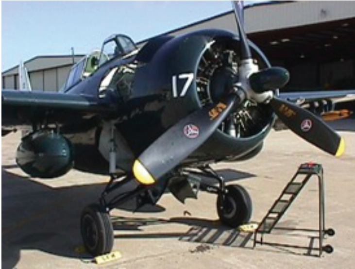
Figure 2. FM-2 Wildcat with Drop Tank (below wing). Photo credit: Cavanaugh Flight Museum
